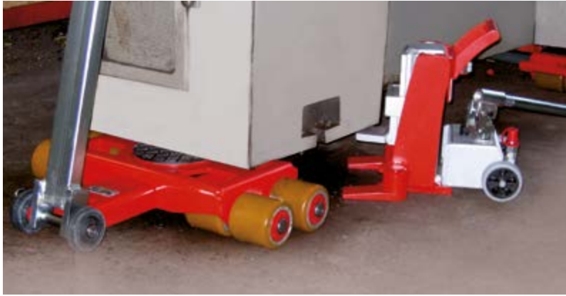
Castors with ball bearings guarantee easy movement.
